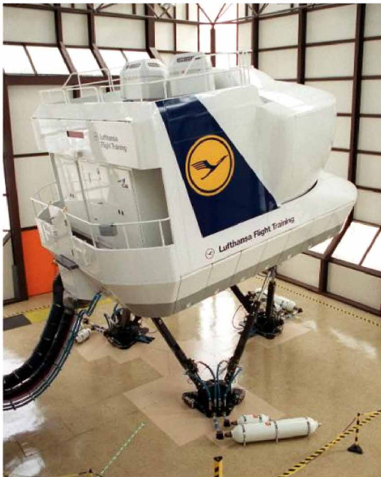
Motion generator for flight simulators
