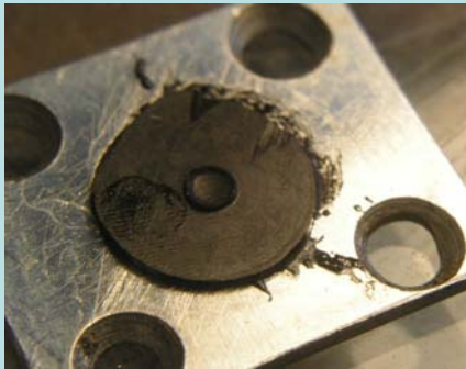
View of hardened NT/epoxy composite tablet with anisotropic conductivity (MIET, 2005)
