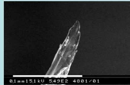
SEM image of Pt/Ir - probe (MIET, 2005)
