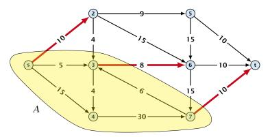
The capacity of the cut is  $cap(A, V \setminus A) = 28$ .
